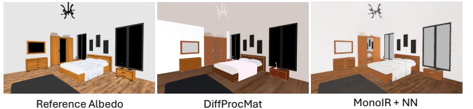
Fig. 7. Mirror region failures. All baselines struggle with mirrors. In this scene from the Bitterli dataset, for the mirror on the closet, DiffProcMat assigns a median color and MonoIR produces a “baked in” appearance.
